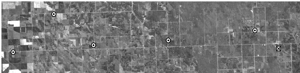
Fig. 5. Prototype sensorweb deployment (five nodes and base station) in Red River flood forecasting context, Manitoba, Canada. Landsat-7 image width is approximately 45 km.
