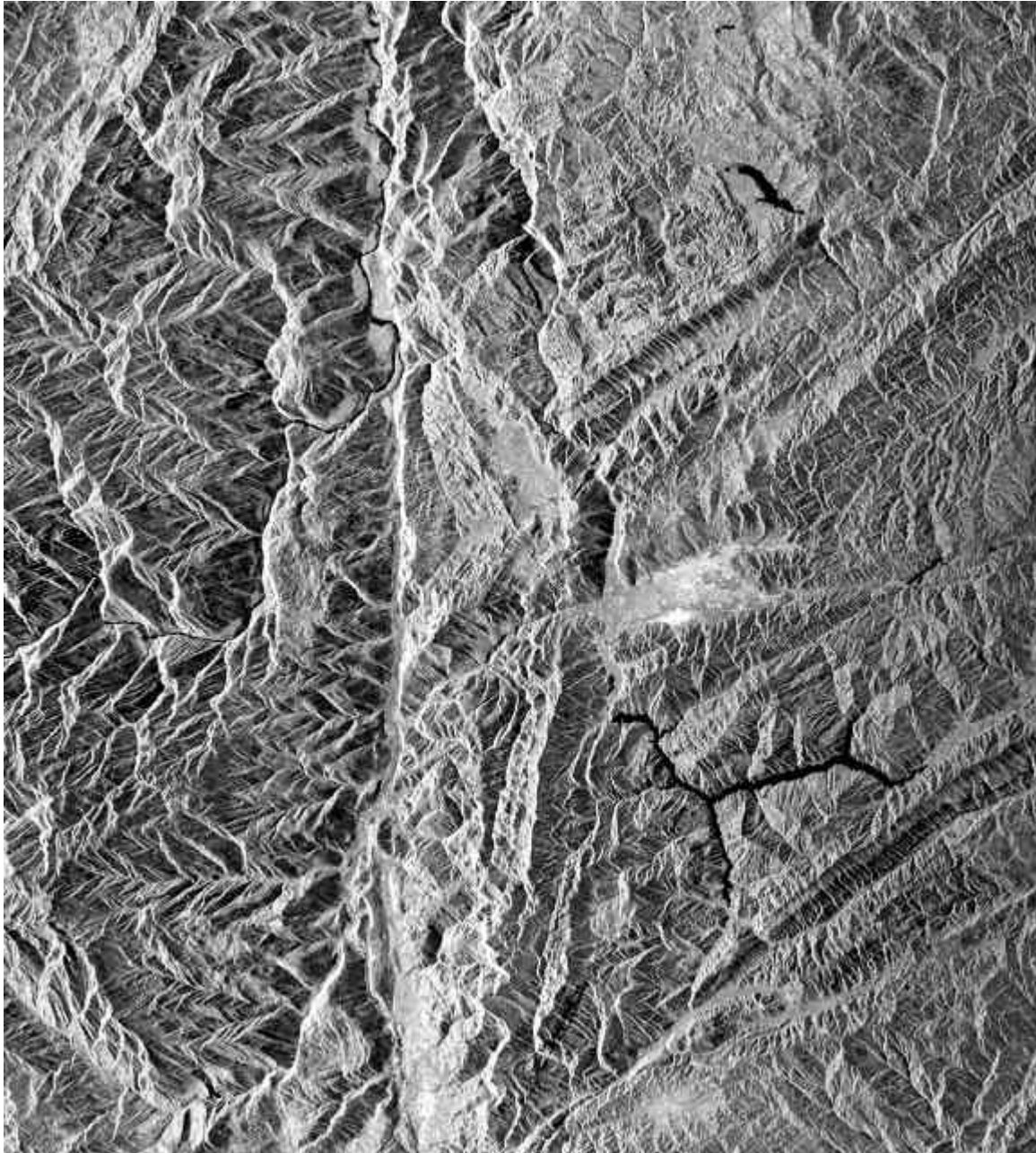
Fig.3 RADARSAT-1 image in the Jinshajiang river area, central Yunnan province, southwestern P. R. China Asc. Orbit, 23-Oct-96, Fine mode, beam3, Incidence angle: 41°-44°, Resolution: 8m.
