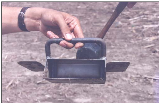
Figure 5. Custom Designed Shovel Used For 5 cm Soil Fertility Sample
