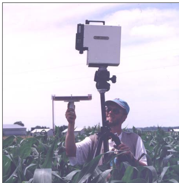
Figure 9. GER3700 Field Spectroradiometer And White Reflectance Spectralon Panel
