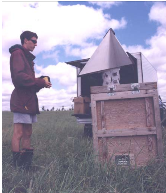
Figure 12. Corner Reflectors Deployed During The Airborne SAR Acquisitions
