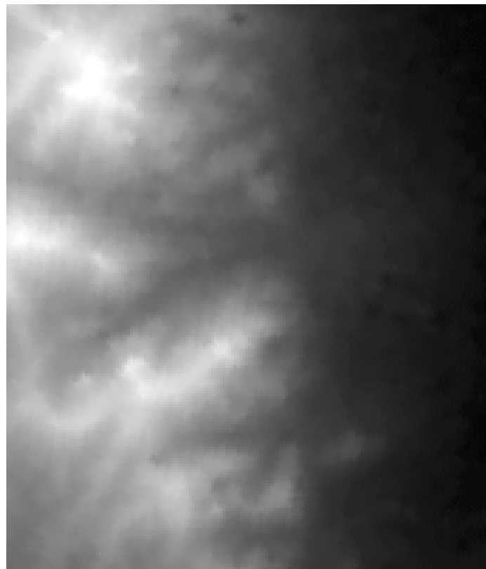
Figure 2: An ASTER-extracted DEM at 30-m spacing
