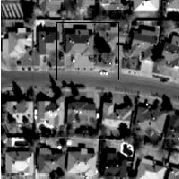
Figure 1: Sub-image (200 x 200 pixel; 61-cm pixel spacing) of Quickbird image acquired over Reno, USA. Courtesy and copyright of DigitalGlobe, 2002
