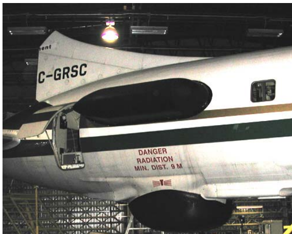
Fig. 1. Tail section of Convair –580 showing SAR radomes.
