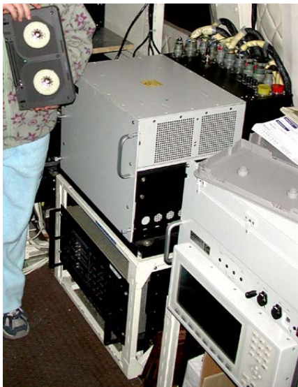
Fig. 2. Recording system. The formatter and verification unit is at the front at the bottom.
