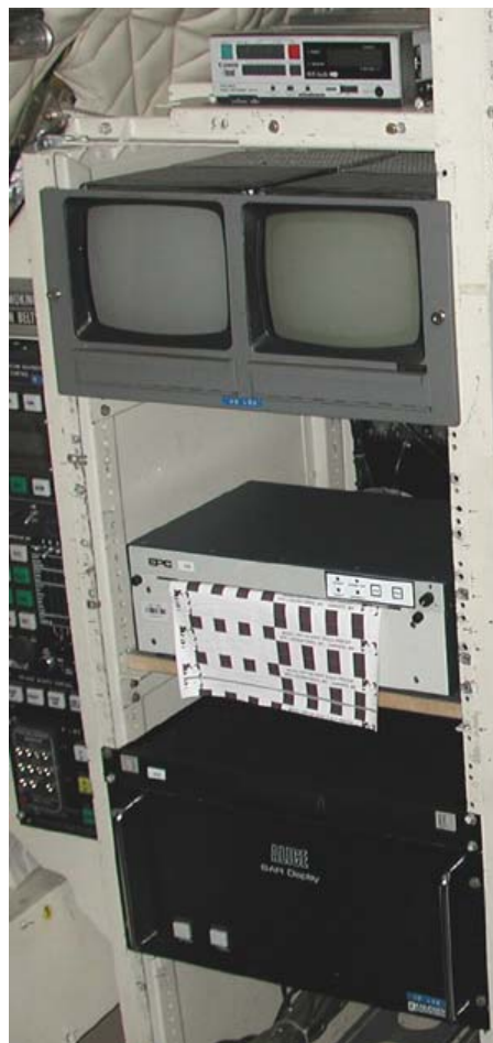
Fig. 3. Real-time image display and printer. At the top are scrolling full-image and blow-up screens. The new printer and display/formatter are below.
