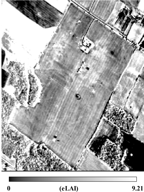
Figure 2: eLAI map of a white bean field derived from Probe-1 hyperspectral reflectance data.
