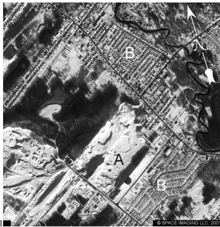
Figure 2: Sub-image of left IKONOS stereo pair, north of Québec City, Quebec, Canada. Note: (A) sand/gravel pits in operation and (B) residential and urban areas. IKONOS Image © Space Imaging LLC, 2001
