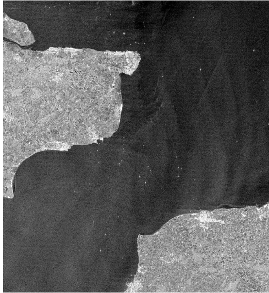
Figure 3.7.2-1 A RADARSAT-1 ScanSAR Narrow Far image of the Straits of Dover. The image covers 76 km from left-to-right. Many bright, point-like ship target signatures are visible in the busy shipping lanes. (©CSA 1997)
