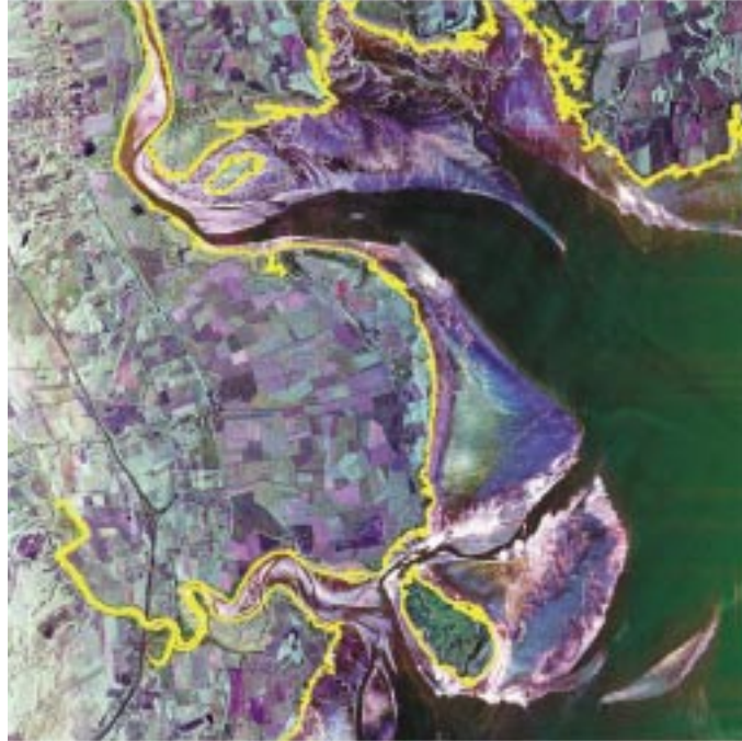
Figure 3.7.5-1 Convair-580 SAR multi-polarization composite of the Minas Basin, N.S. during low tide conditions. The HH, HV, and VV polarized images are shown in red, green and blue, respectively. The yellow line marks the boundary between the dry land and the tidal plane. The backscatter contrasts in these two areas were enhanced independently to produce the image shown. The colourful patterns present illustrate the differences in the information content of the three images.
