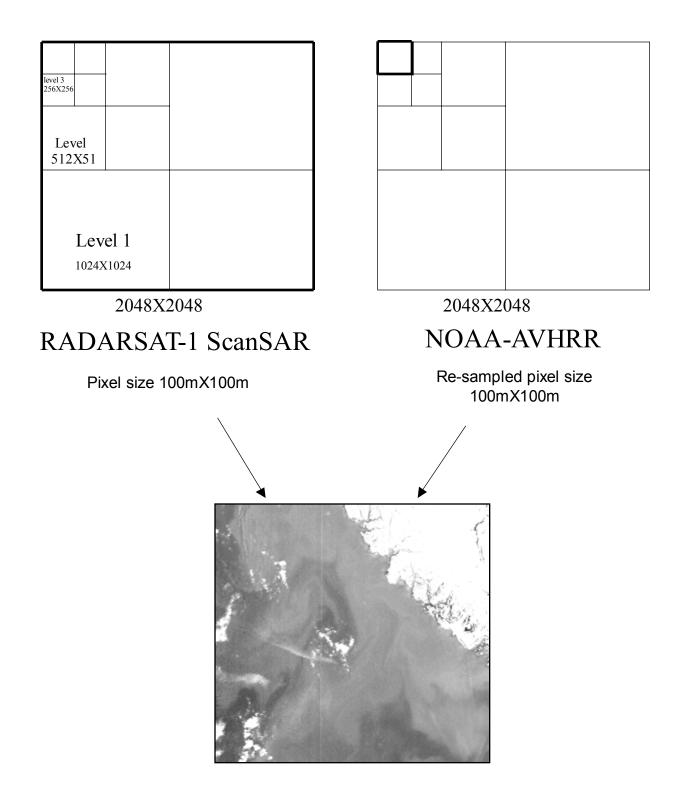
**Figure 2**. Conventional image fusion by using the wavelet transform. The NOAA-AVHRR image is resized from 256×256 pixels to 2048×2048 pixels using bilinear interpolation, and the pixel size from 800m by 800m to 100m by 100m.
