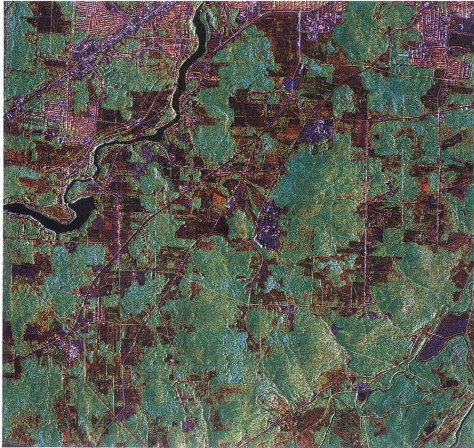
Figure 4: Composite ortho-images (10 by 10 km; 5-m pixel spacing) using IHS radiometric coding with SAR-west in I, SPOT-P in H and SAR-east in S.
