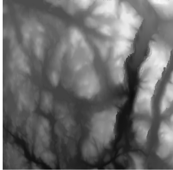
Figure 4. DEM corresponding to the image of Fig. 3. Geometric distortions in the image result from the combination of view direction and the local slope.
