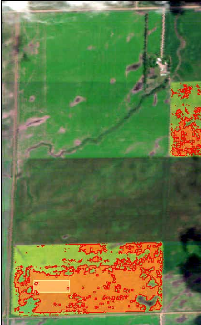
Figure 4: Agricultural scene with canola training set identified by a yellow rectangle and pixels classified using the default threshold value identified by red pixels. The RGB image was generated using bands centered at 676.3 nm for red, 540.5 nm for green, and 478.8 nm for blue.
