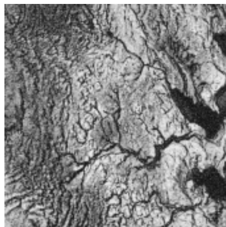
Fig. 3 a) Interferogram-magnitude, b) "Flat earth" corrected phase, and c) Scene coherence. One phase cycle represents a relative change in elevation equal to 21 m.
