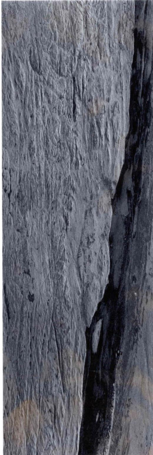
Figure 1: RADARSAT-SAR image (6590 pixels by 19172 lines) of the Charlevoix region: descending orbit, standard beam (S2), slant range (8.1 m by 5.3 m), satellite track oriented. Illumination direction is approximately from west to east. © CSA/ASC 1996
