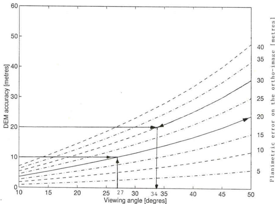
Figure 2: Relationship between the RADARSAT-SAR image acquisition viewing angle (degrees), the DEM accuracy (metres) and the planimetric error on the ortho-image (metres). The arrows and the solid curves represent numerical examples of the relationship between the three parameters.
