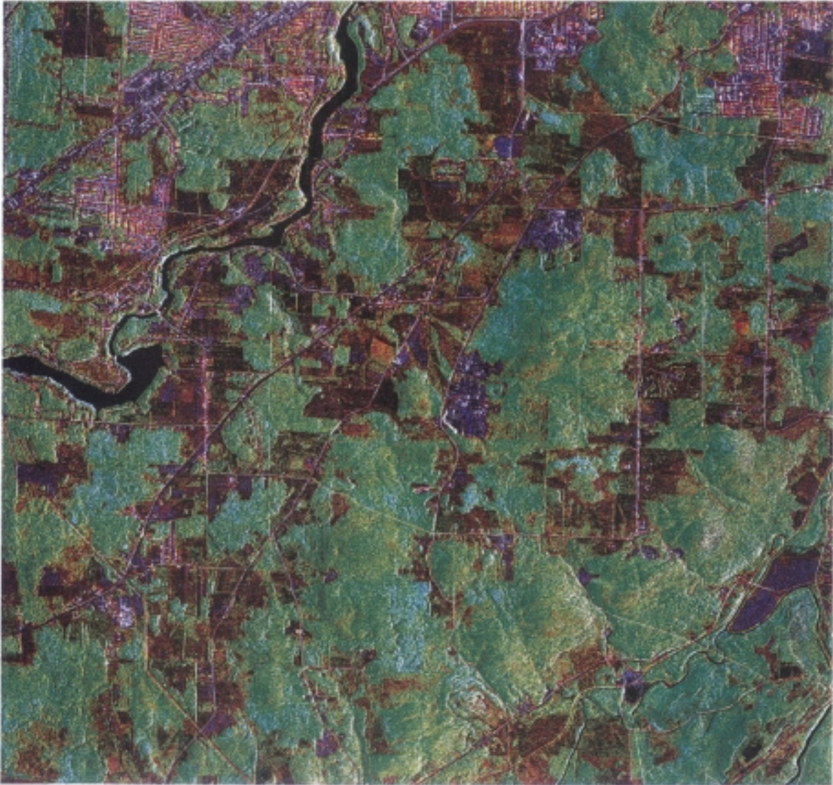
Figure 6: Enlargement of a colour composite ortho-image of SPOT-PLA and two airborne SAR (10 km by 10 km; 5-m pixel spacing)
