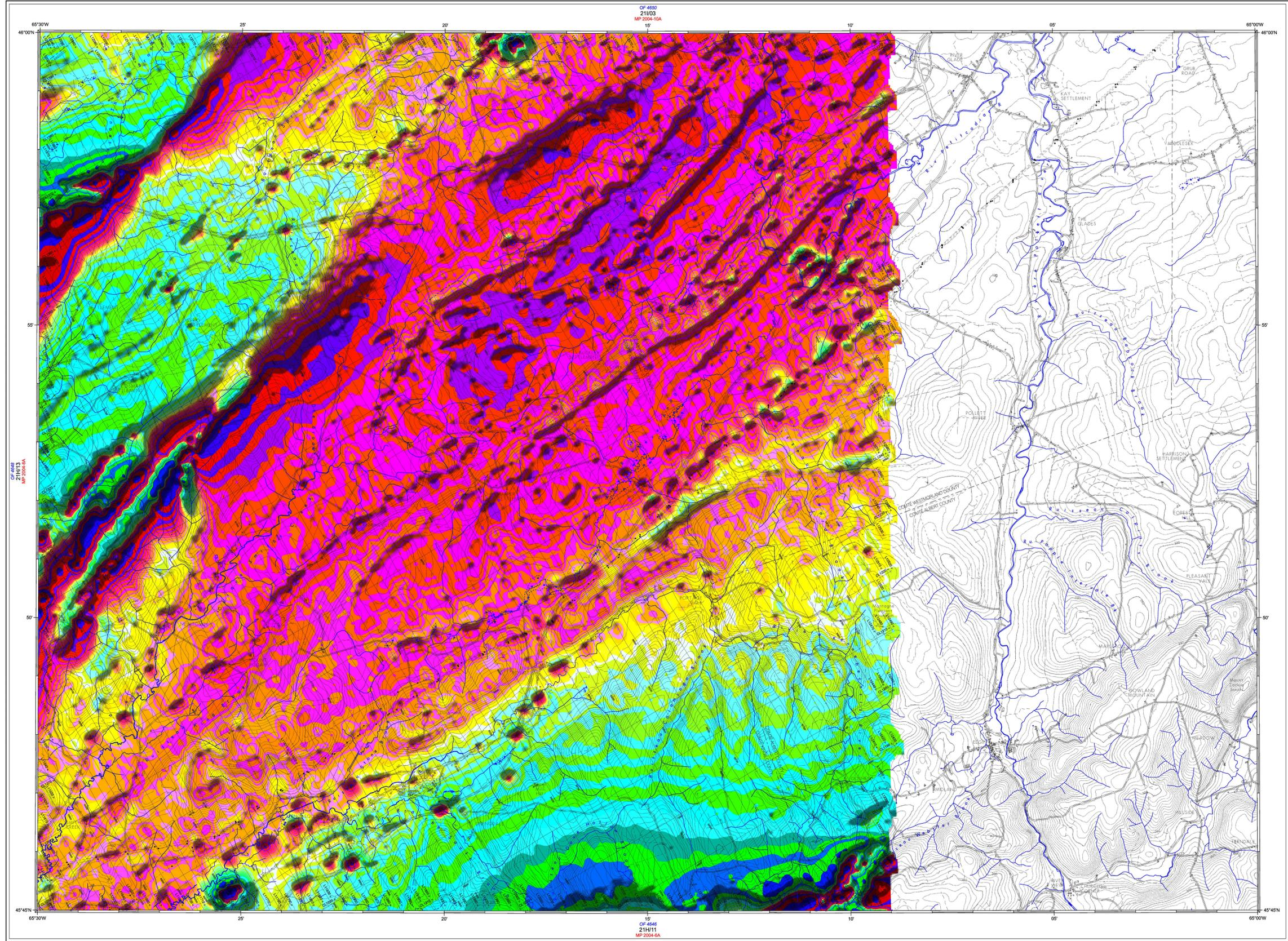
This map was compiled from data obtained as a result of an aeromagnetic survey carried out by Sander Geophysics Limited using a Cessna Grand Caravan (registration C-GSGW) aircraft. A 0.05 T sensitivity cesium vapour magnetometer was mounted in the tail boom of the survey aircraft.
