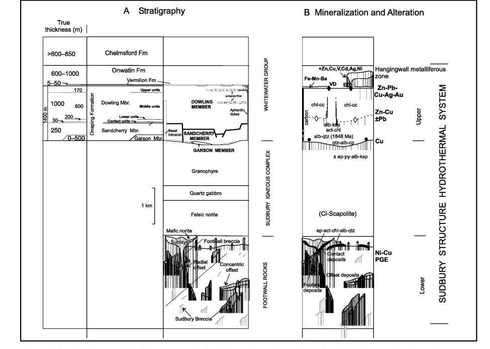
Figure 2. Schematic sections through the Sudbury structure showing: A) Stratigraphic terminology with member and unit thicknesses. The fragmental rocks are intruded by fine grained aphanitic dykes and the xenolithic basal intrusion; B) Distribution of mineralization and alteration, Sudbury structure hydrothermal system. VD, ED = Vermilion and Errington Zn-Pb-Cu-Ag deposits. (Modified after Ames et al., 2002).
