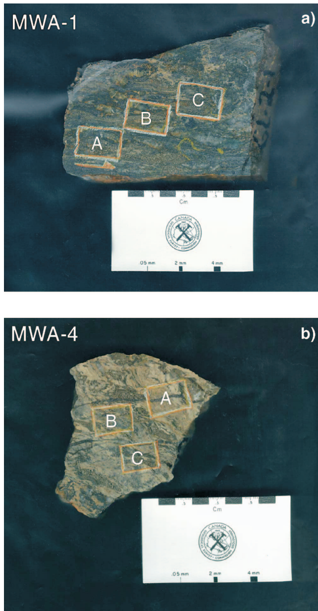
Figure 1. Images of the slabs selected for this study. The locations selected for subsamples are labelled A, B, and C for samples a) MWA-1 and b) MWA-4.
