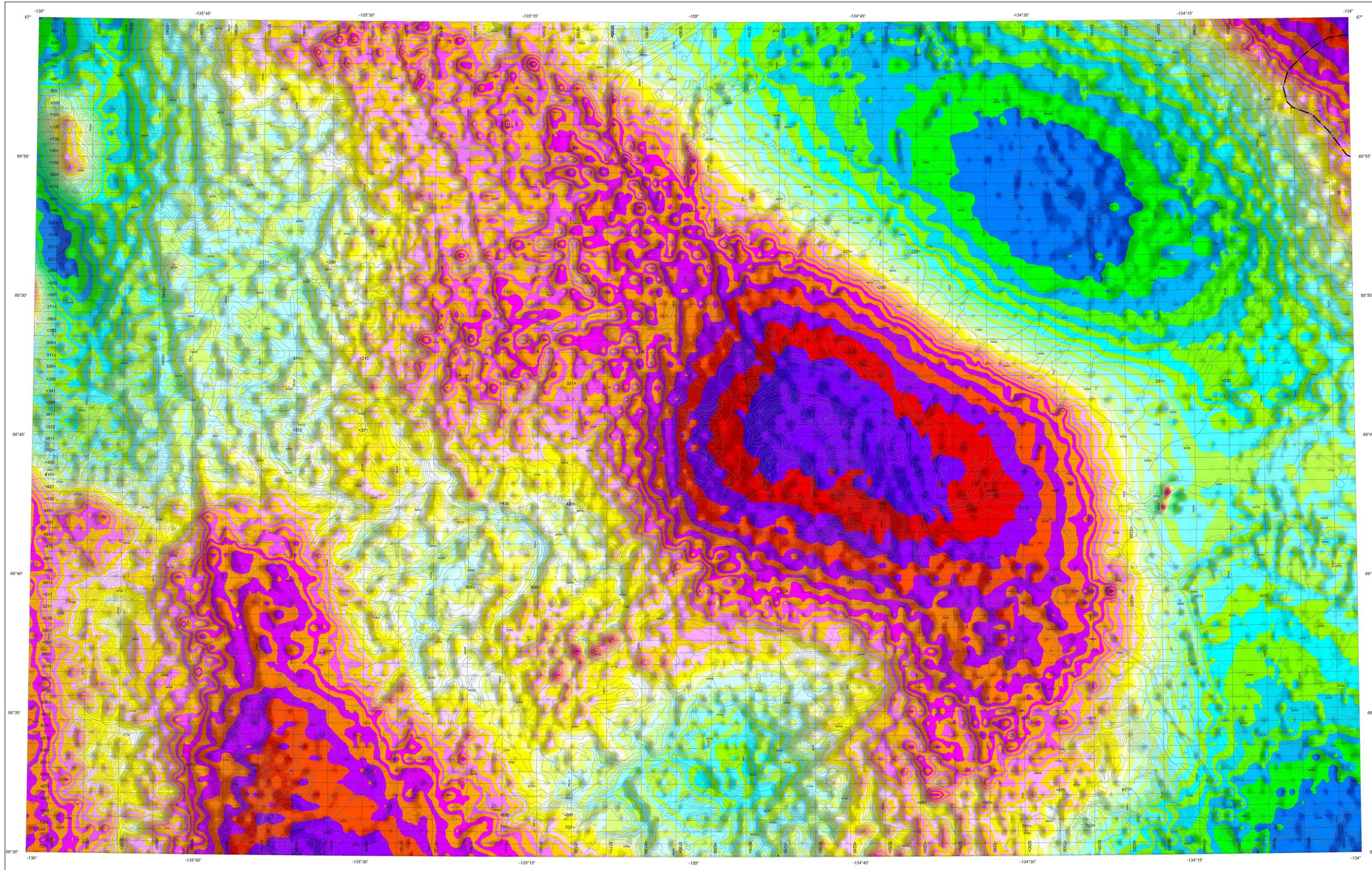
This map was compiled from data obtained as a result of an aeromagnetic survey carried out by Fugro Airborne Surveys using a Cessna Caravan (registration C-FZLX) aircraft. A 0.005 nT sensitivity split-beam cesium vapour magnetometer was mounted in the tail boom of the survey aircraft.
