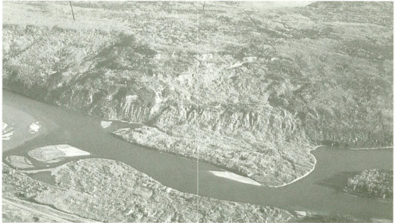
The Attachie landslide occurred suddenly in the night of May 26, 1973, along the Peace River 88 km west of Fort St. John, B.C. The landslide involved 12.4 million cubic metres of fine-grained Pleistocene materials and blocked the Peace River for about 12 hours. Joint work in 1993-94 by the GSC and B.C. Hydro has attempted to establish the geological and geotechnical factors that led to the landslide and to unravel the mechanism by which some of the debris travelled very rapidly over the flat Peace River valley floor over a kilometre from its source.
