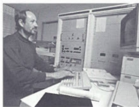
Isotope analysis using a solid source mass spectrometer
