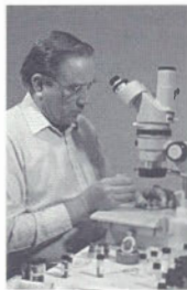
Selecting zircon grains to undergo age determination
