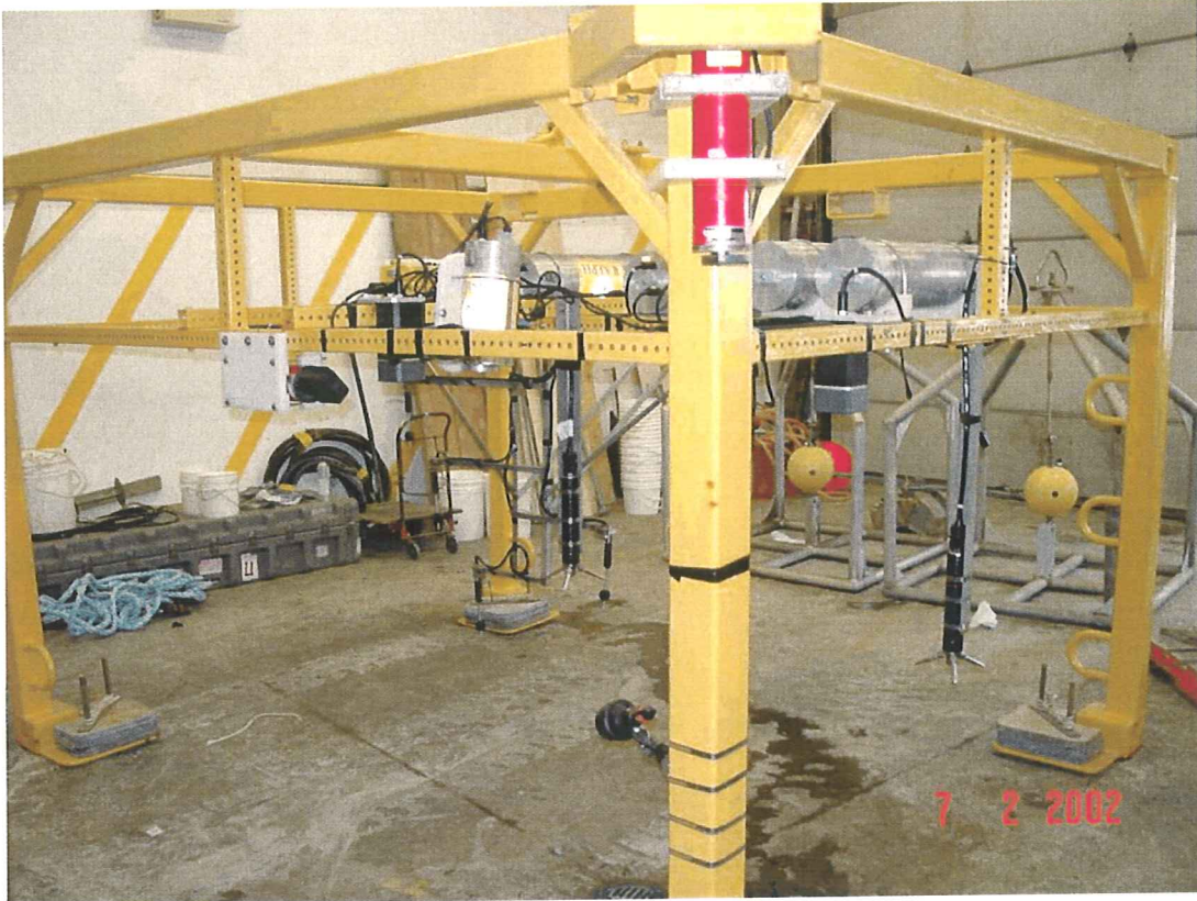
Fig. 5-1 An image of the recently upgraded GSC instrumentation platform RALPH with S4 current meters in the background.
