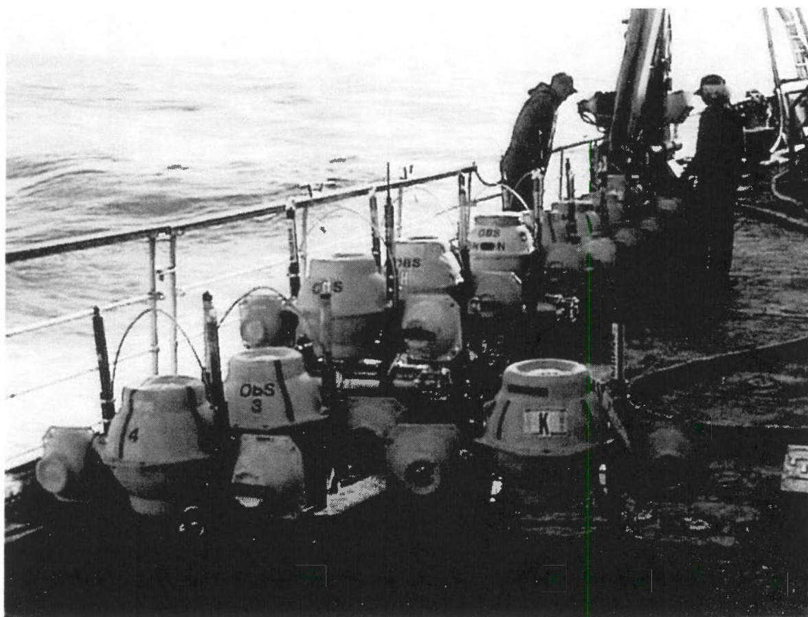
Figure 3. Bob and Walter preparing OBS for deployment on the starboard waist.
