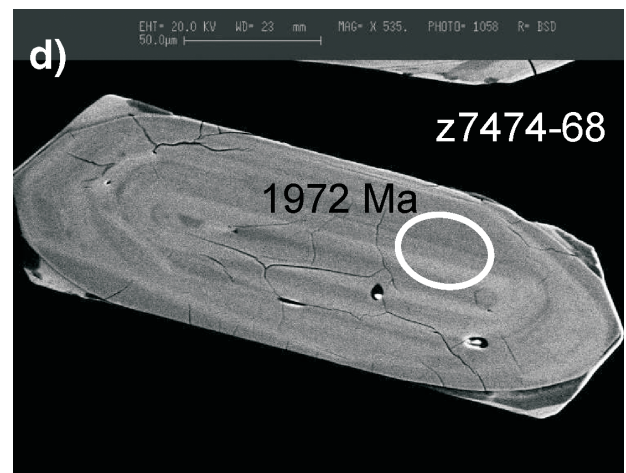
Figure 3. Zircons from z7474, aplitic granite, Virgin River shear zone; a) transmitted light, b)–d) back-scattered electrons. Ellipses show locations of SHRIMP analysis sites and ^{207}\text{Pb}/^{206}\text{Pb} dates.
