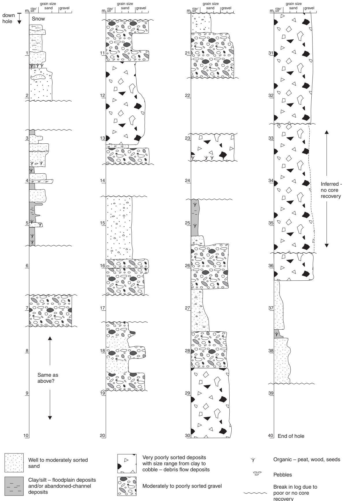
Figure 3. Drill log for hole DHPV09. The vertical axis shows the depth of the hole below the surface, and the horizontal axis shows the average grain size of the sediment layers.
