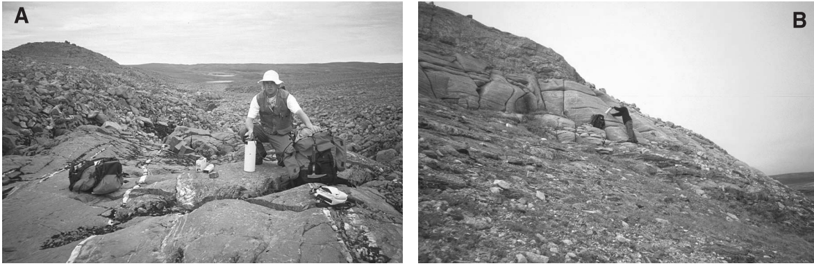
Figure 1. Ground gamma-ray spectrometry measurements on A) psammite of the Longstaffe Bluff Formation and B) marble of the Flint Lake Formation, lying between high-potassium calc-silicate unit (top) and muscovite schist (bottom). Both figures show the 2- \pi geometry required for accurate gamma-ray spectrometry measurements.
