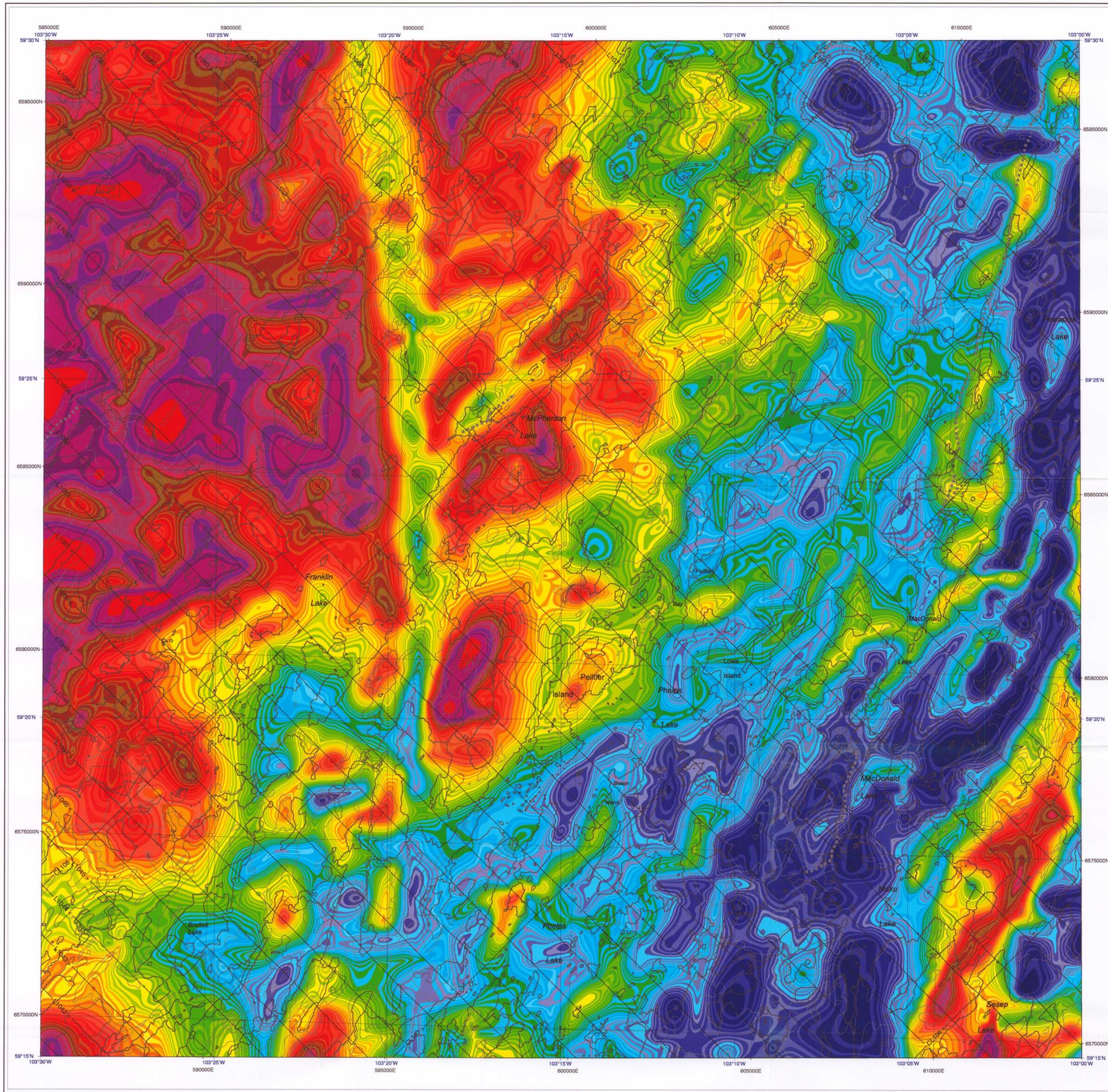
An airborne geophysical survey of the Phelps Lake area, Saskatchewan, was flown by Sander Geophysics Limited (SGL) for the Geological Survey of Canada and Saskatchewan Energy and Mines. The purpose of the survey was to obtain gamma-ray spectrometric, aeromagnetic and VLF-EM data. The survey was flown between August 14 and September 7, 2000 using a Bristow-Norman Islander (BN22-1) aircraft flying 120 m above the terrain at a mean speed of 220 km/h.
