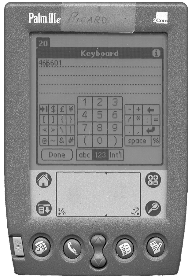
Figure 3. The on-screen touch-sensitive keypad used for numerical data entry.
