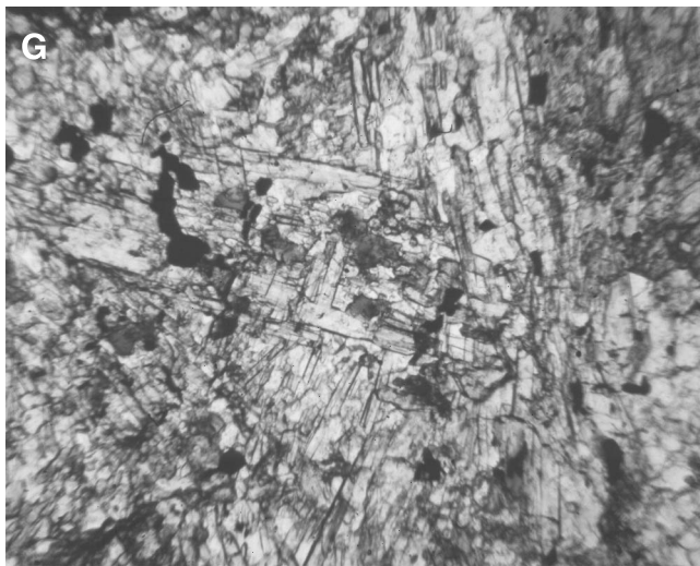
Figure 3. E ) thinly banded rhyolite tuff (west central Aylmer dome); F ) gossanous weathering of silicate-sulphide facies iron-formation; G ) photomicrograph of silicate iron-formation showing abundant white amphibole (grunerite) and minor pyrite (40x magnification).
