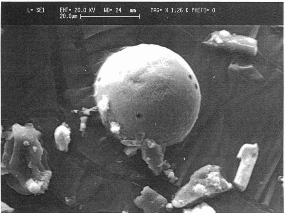
Figure 3: Print #S02-03. A sphere composed of Cu and S. Most likely smelter derived. Note the pockmarks on the surfaces and its texture.
