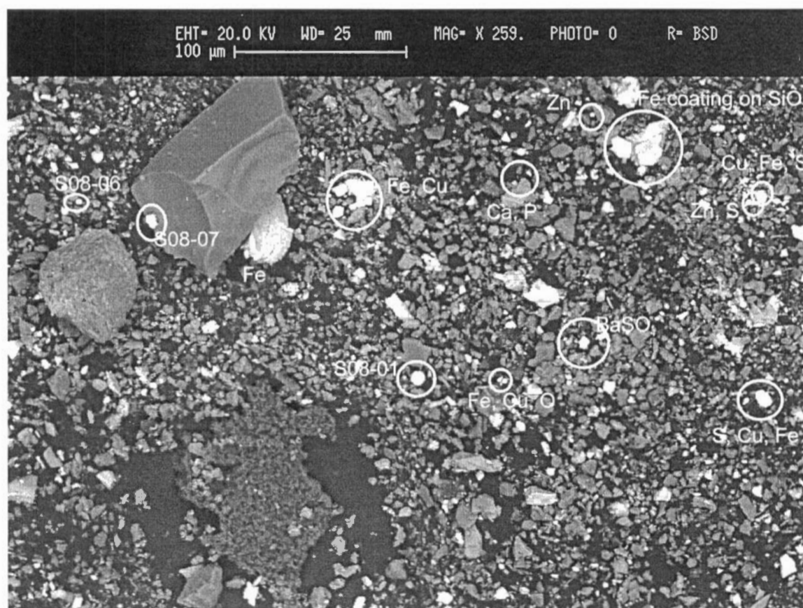
Figure 12: Print #S08-02. An overview of sample S08 which is extremely rich in metals, especially Fe, Cu, S and Zn. Particulate is angular and size variable with large grains like plagioclase, small shavings of Fe-oxide, barite, apatite, quartz, K-spar, native Zn, chalcopyrite, and sphalerite.
