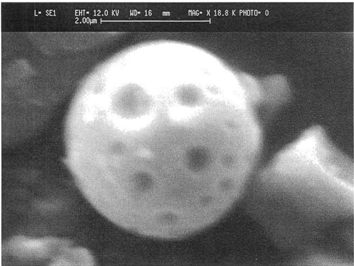
Figure 16: Print #S08-06. Close up of the S, Cu, Fe sphere displaying a pockmarked surface or a "Swiss cheese" texture.
