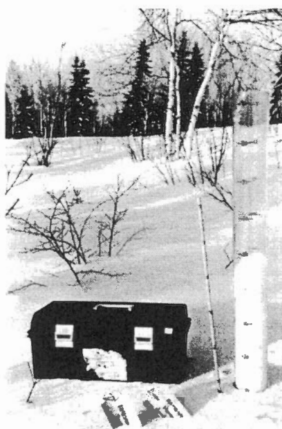
Figure 8 (right): A photo of the PC snow corer, metre stick, sample tags and 16L toolbox for scale. The inside core diameter is 9.0 cm.
