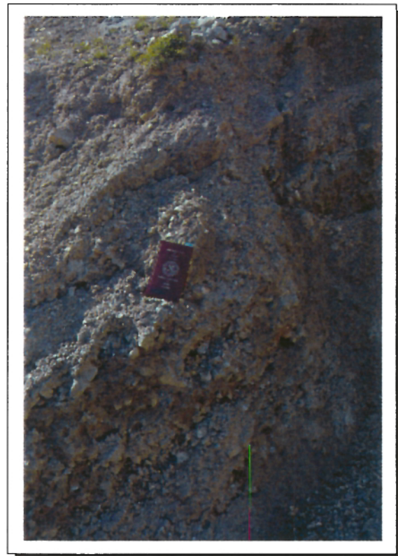
Figure 4.7 Close-up of the colluvial material eroded during the debris flow by a tributary on the eastern slope of the Five-Mile Creek valley. Sample #1 was taken in this deposit at elevation 2100 m. The material is mostly pebble, gravel, with sand and silt. See Figure 4.3 for location of the photograph. A field book gives the scale.
