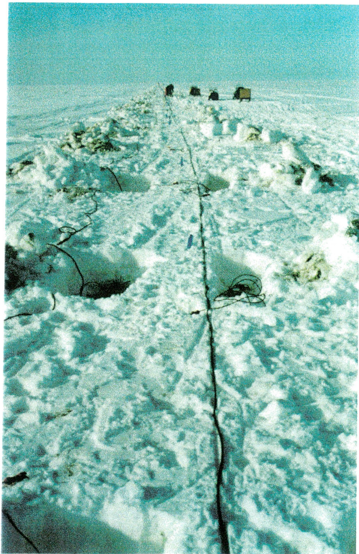
Figure 8: Parallel strings of Mark Products L28A, 30 Hz phones and L28E, 40 Hz phones deployed for comparison purposes.
