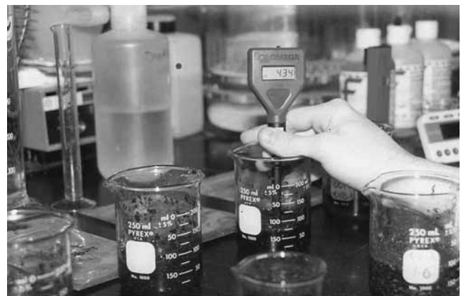
Figure 2. The Omega PHH-7X pen was used to determine the pH of samples in both field and laboratory measurements.
