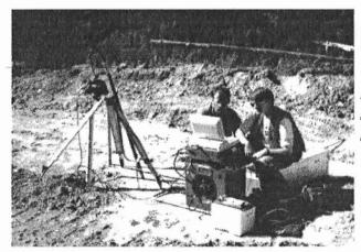
**Figure 4-1.** Geonics EM-39 borehole logging system (gamma, conductivity, magnetic susceptibility sondes) in field use.
