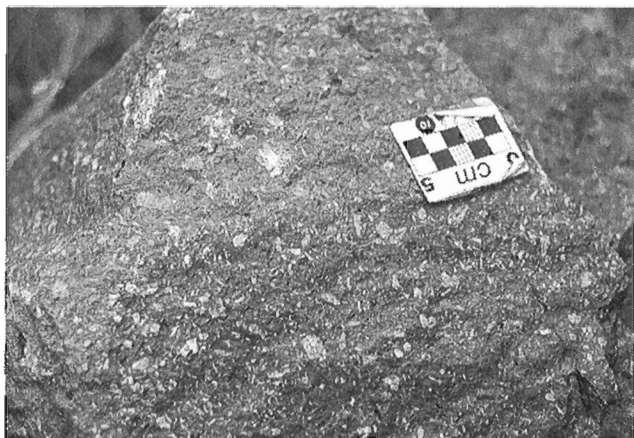
Figure 7. Plagioclase-phyric texture in basalt at Macdonald Rock Pit locality. White phenocrysts of plagioclase are 1 cm in long dimension.
