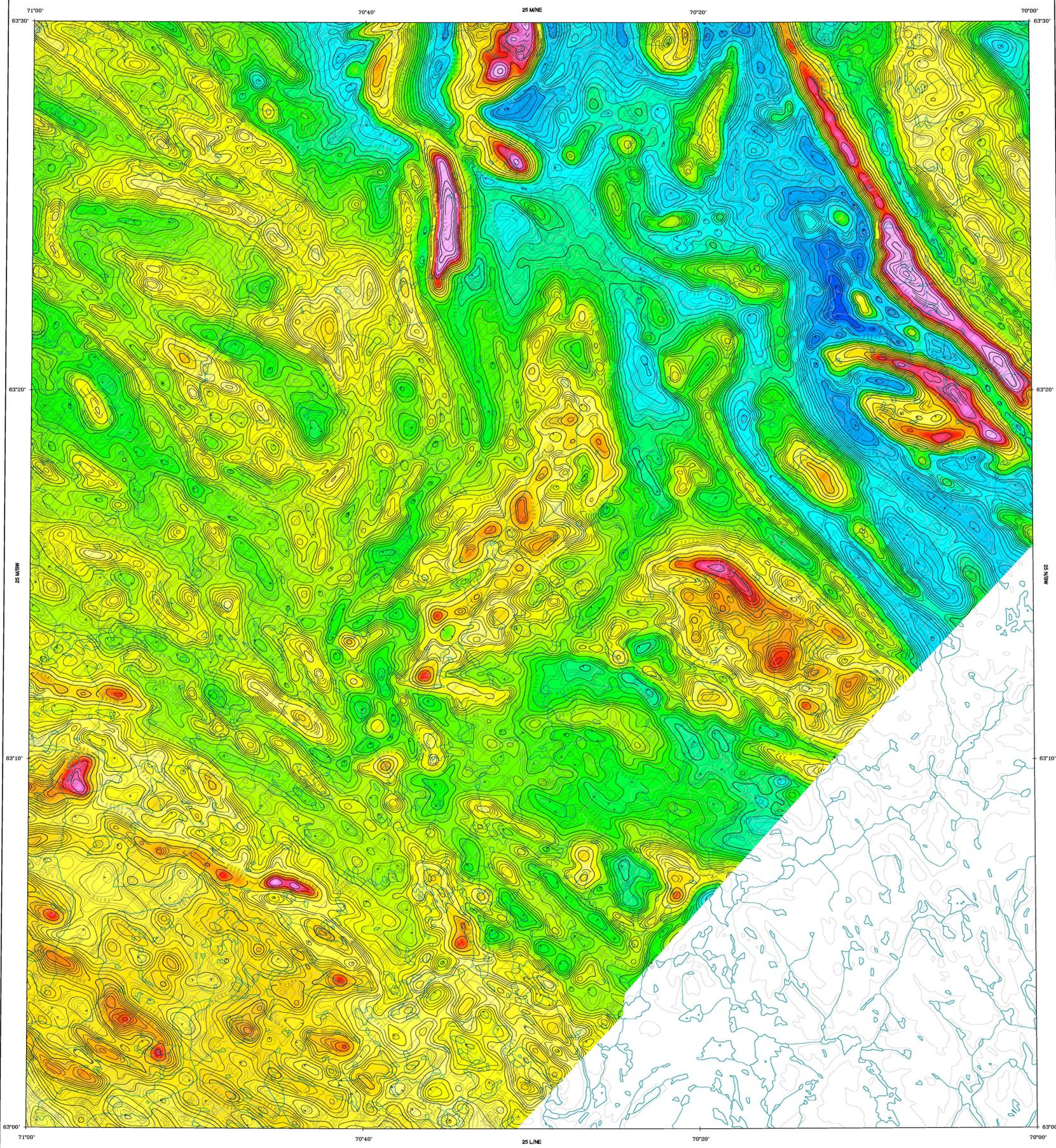
This map was compiled from data obtained as a result of an aeromagnetic survey carried out by SIAL Geosciences Inc. using a NAVALJO 310 aircraft (registration C-GYTT) and a CESSNA 337G aircraft (registration C-GJOD). A 0.005 nT sensitivity split-beam cesium vapour magnetometer was mounted in the tail boom of the survey aircraft.
