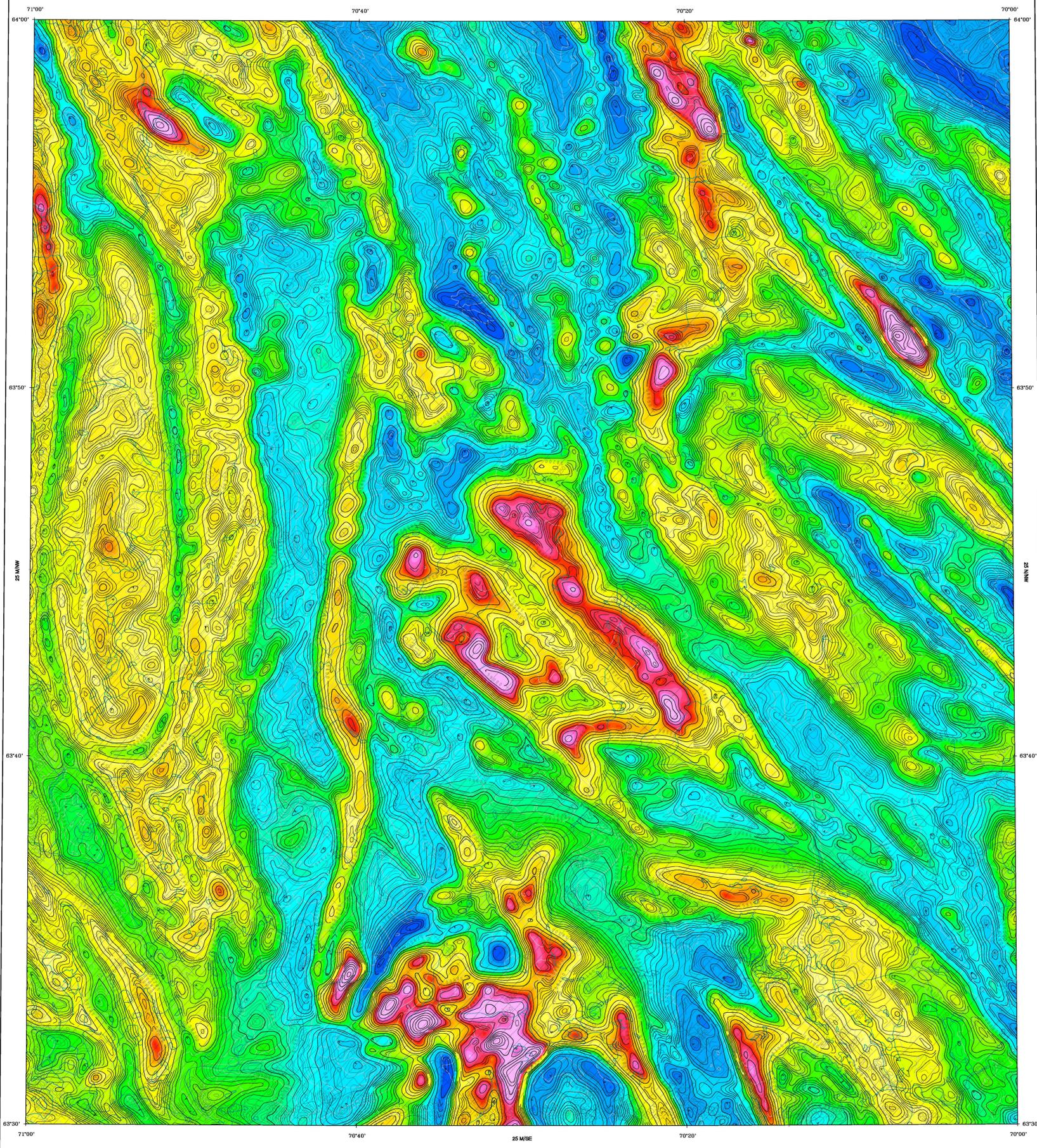
This map was compiled from data obtained as a result of an aeromagnetic survey carried out by SIAL Geosciences Inc. using a NAVAJ0 310 aircraft (registration C-GYTT) and a CESSNA 337G aircraft (registration C-GJOD). A 0.005 nT sensitivity split-beam cesium vapour magnetometer was mounted in the tail boom of the survey aircraft.
