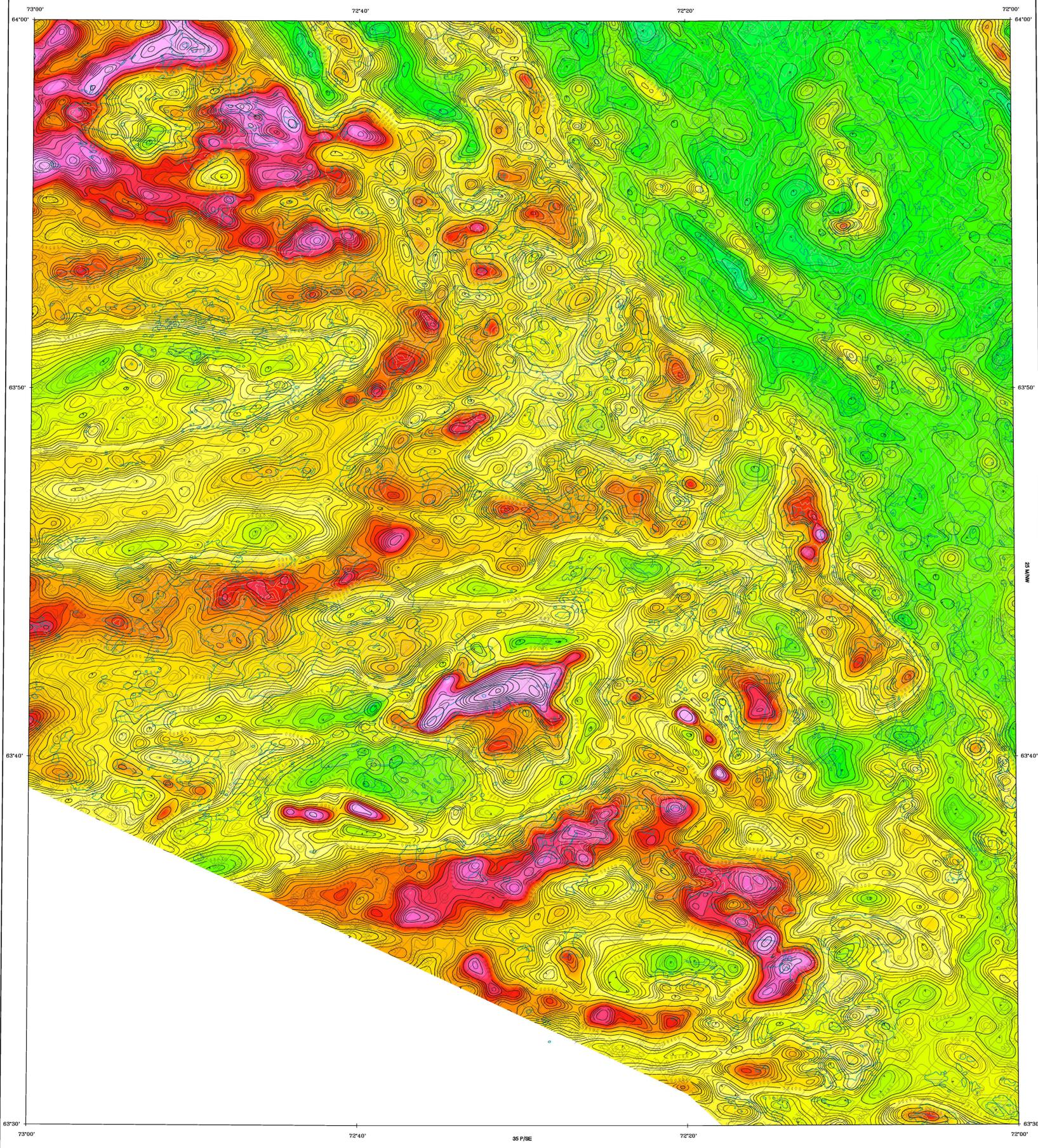
This map was compiled from data obtained as a result of an aeromagnetic survey carried out by SIAL Geosciences Inc. using a NAVAJO 3D aircraft (registration C-GYTT) and a CESSNA 337G aircraft (registration C-GJOD). A 0.005 nT sensitivity split-beam cesium vapour magnetometer was mounted in the tail boom of the survey aircraft.
