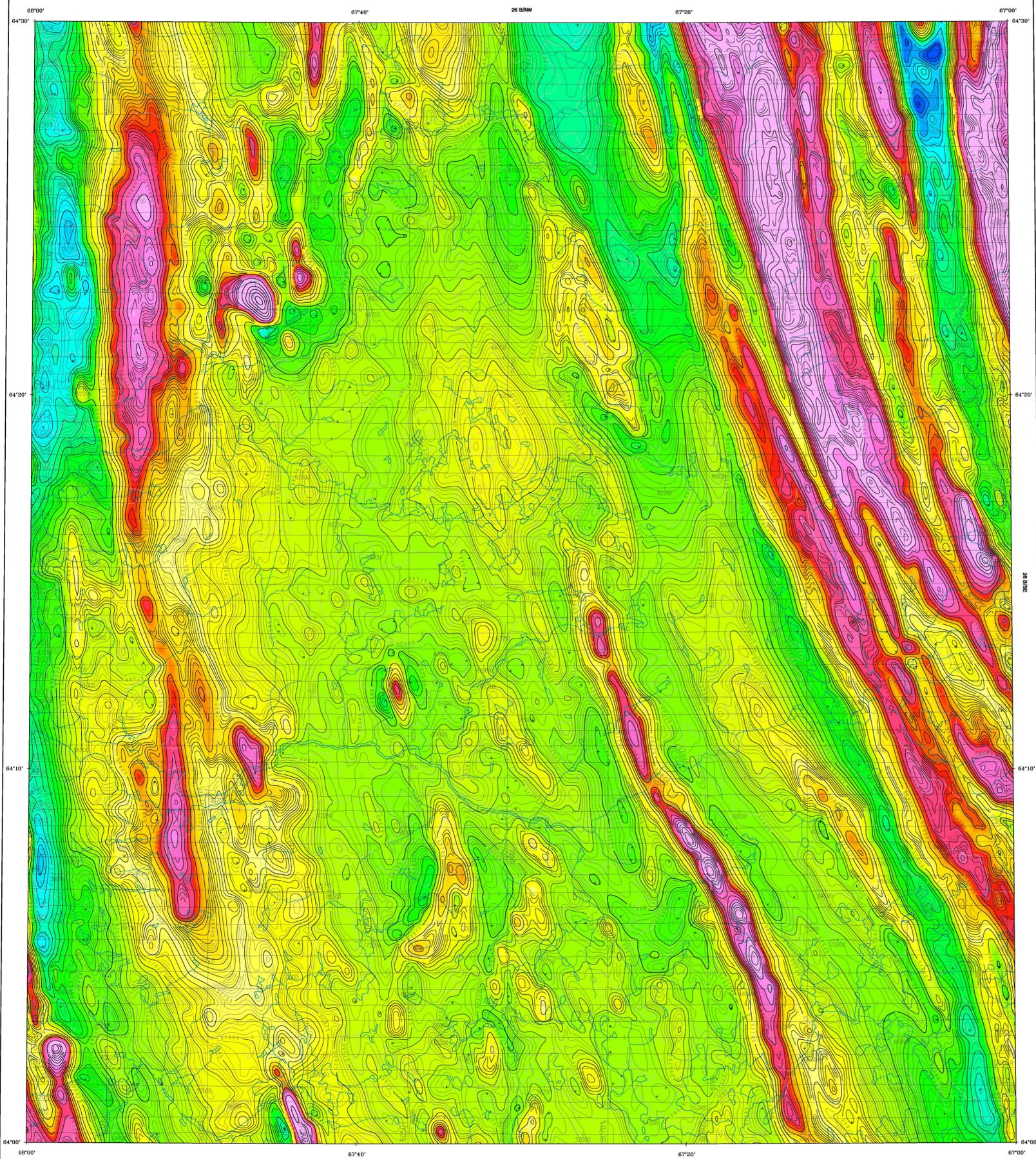
This map was compiled from data obtained as a result of an aeromagnetic survey carried out by SIAL Géosciences Inc. using a NAVAJO 310 aircraft (registration C-GYTT) and a CESSNA 337G aircraft (registration C-GUJD). A 0.005 nT sensitivity split-beam cesium vapour magnetometer was mounted in the tail boom of the survey aircraft.
