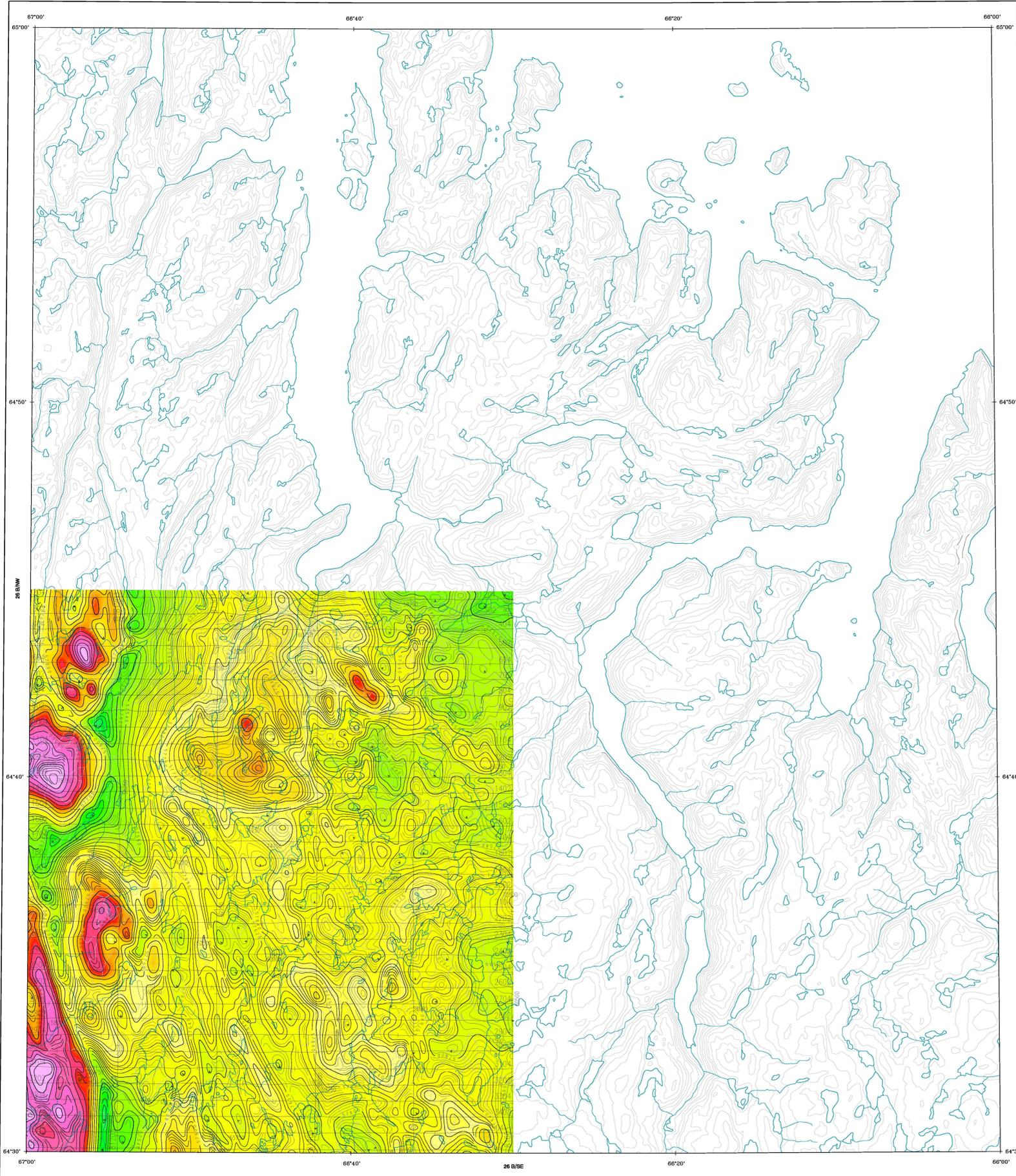
This map was compiled from data obtained as a result of an aeromagnetic survey carried out by SIAL Geosciences Inc. using a NAVAJO 3D0 aircraft (registration C-GYTT) and a CESSNA 337G aircraft (registration C-GJOD). A 0.005 nT sensitivity split-beam cesium vapour magnetometer was mounted in the tail boom of the survey aircraft.
