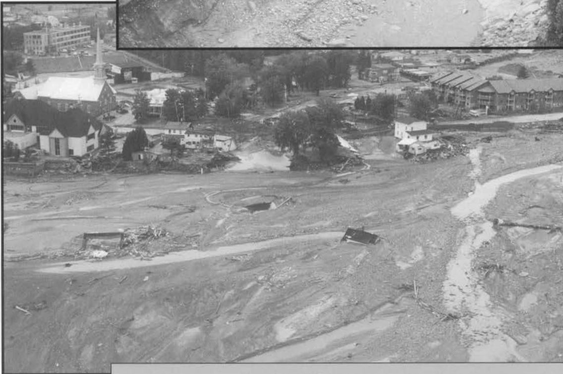
Figure 23. At the mouth of the Ha! Ha! River, sediment and debris eroded by floodwaters upstream were carried out onto and aggraded the tidal flats (foreground), greatly increasing the subaerial extent of the flats, especially at low tide. As a striking example of the power of this flood, a bank located at the river mouth within the city of La Baie was destroyed during the flood and its 35 tonne safe was carried about 300 m out onto the tidal flats (Plan, 1996). The safe was located about three weeks later. Photograph taken on July 25, 1996. (GSC 1998-015G)
