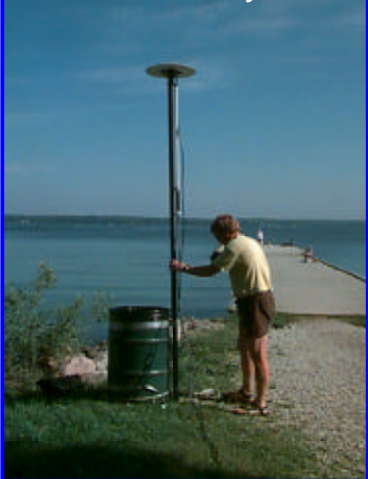
Setting up base station on shore for DGPS system.
