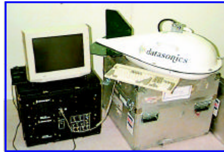
Datasonics Chirp II subbottom profiler (sonar sweep 2-7 kHz)
