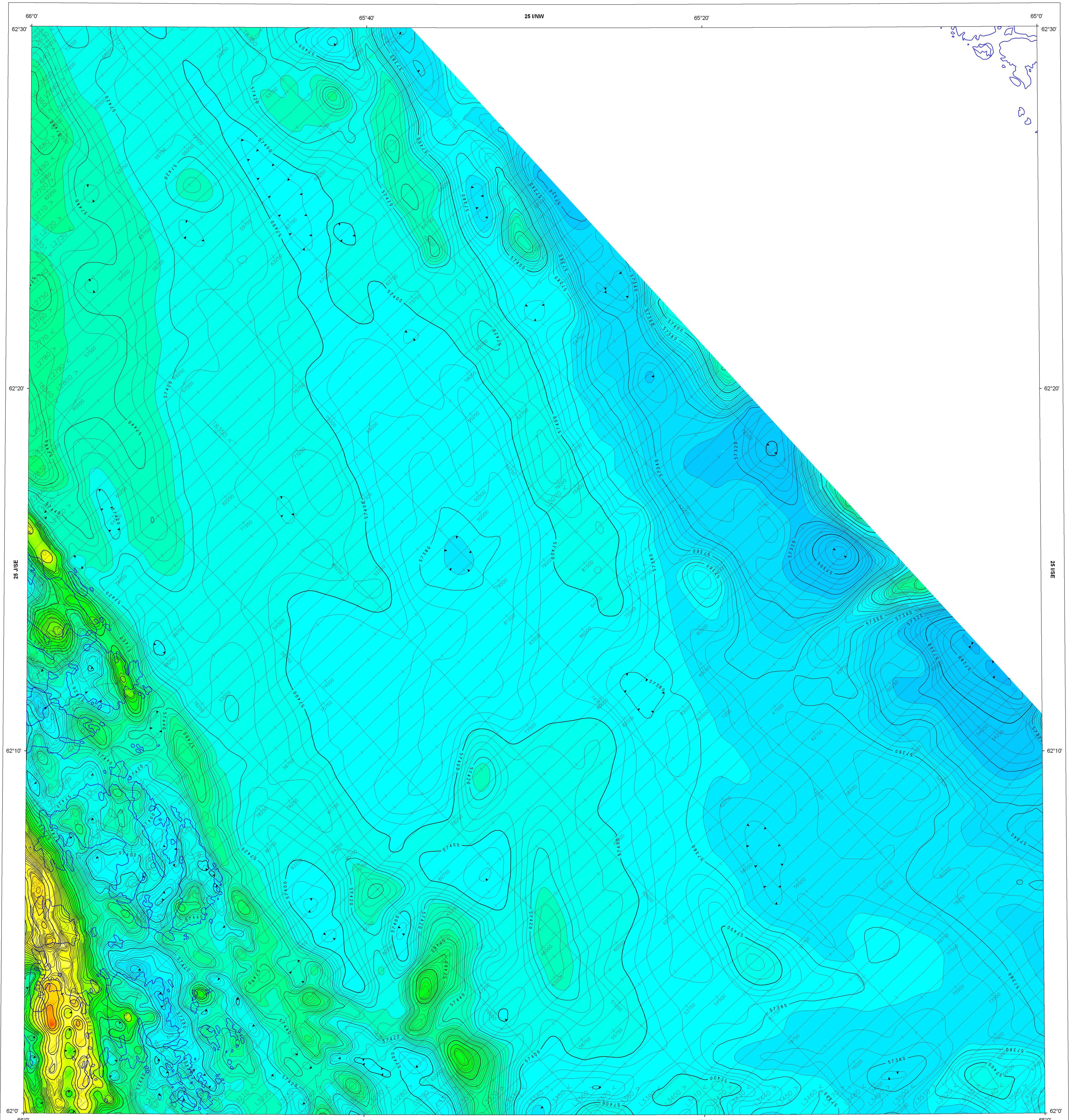
This map was compiled from data obtained as a result of an aeromagnetic survey carried out by Goldak Exploration Technology Ltd., using a Cessna 337 (registration C-GQD) and a Piper Navajo (registration C-FJBA) aircraft. A 0.005 nT sensitivity split-beam cesium vapour magnetometer was mounted in the tail boom of the survey aircraft.
