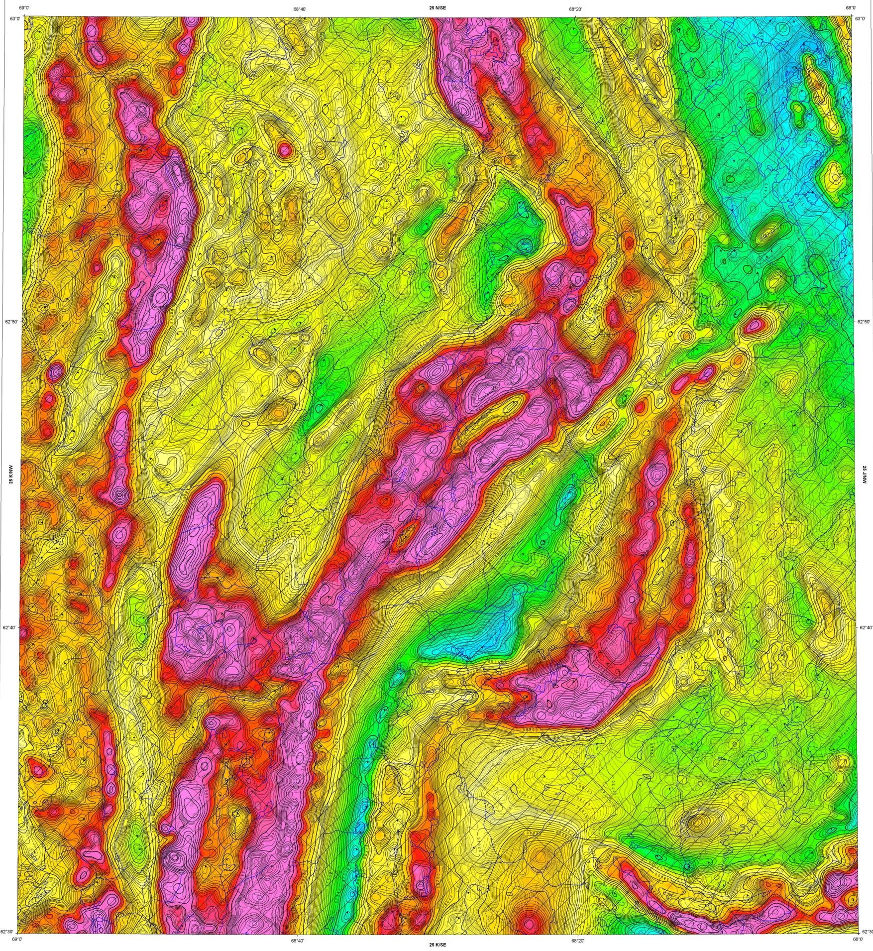
This map was compiled from data obtained as a result of an aeromagnetic survey carried out by Goldak Exploration Technology Ltd. using a Cessna 337 (registration C-GJOD) and a Piper Navajo (registration C-FJBA) aircraft. A 0.005 nT sensitivity spill-beam cesium vapour magnetometer was mounted in the tail boom of the survey aircraft.
