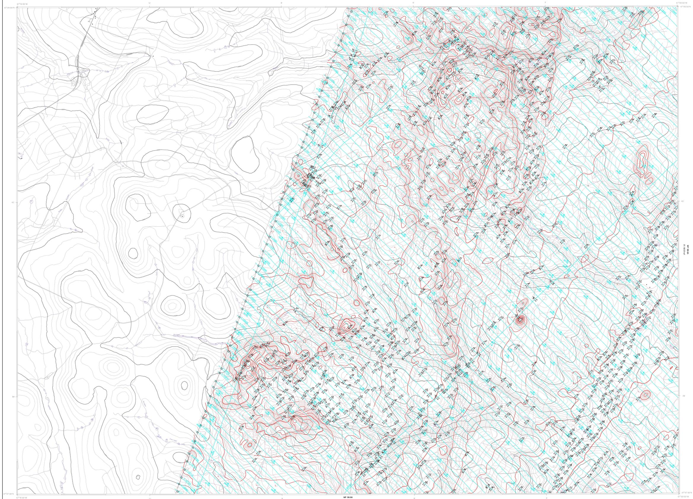
This map was compiled from data acquired during an electromagnetic-magnetic aeromagnetic survey carried out by Aerodat Inc. utilizing an Aeromagnetic AS5000A helicopter (registration C-GJDD). The survey operations were carried out from July 18 to October 6, 1997.
