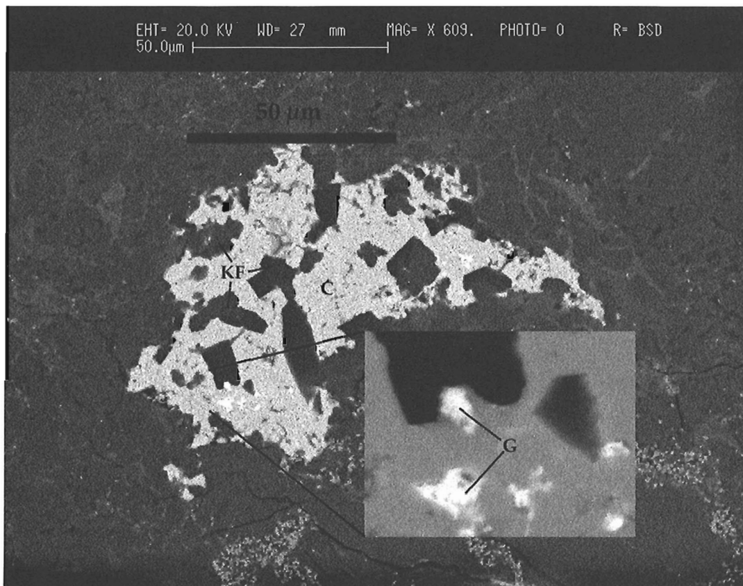
Figure 10. BSE image of a chalcopyrite (C)–potassium feldspar (KF) segregation in the Iron Ridge tuff. Galena (G) is a minor component.
