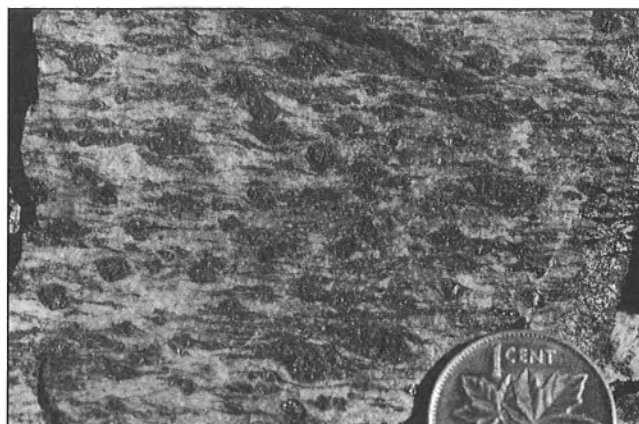
Figure 84. Detail of streaky Mary granite mylonite, Turnbull Lake. The cores of the dark 'studs' are garnets with hornblende rims and tails pulled out along the mylonitic foliation. The winged inclusions formed by the cores and tails indicate sinistral shear in the photograph (upper centre), but this loose block is probably inverted. Note the absence of feldspar porphyroclasts. In thin section, the assemblages are more complex: the cores of garnet are in textural equilibrium with spatially associated orthopyroxene-clinopyroxene and hornblende. The orthopyroxene is more readily replaced by amphibole than is the clinopyroxene. Coin for scale 2.5 cm. GSC 1994-214
