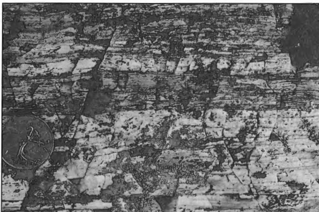
Figure 147. Sheets of leucogranite ribbon mylonite (white) in ribbon mylonite of paragneissic origin, south Snowbird Lake. Note absence of porphyroclasts. Coin for scale 2.5 cm. GSC 1994-210
