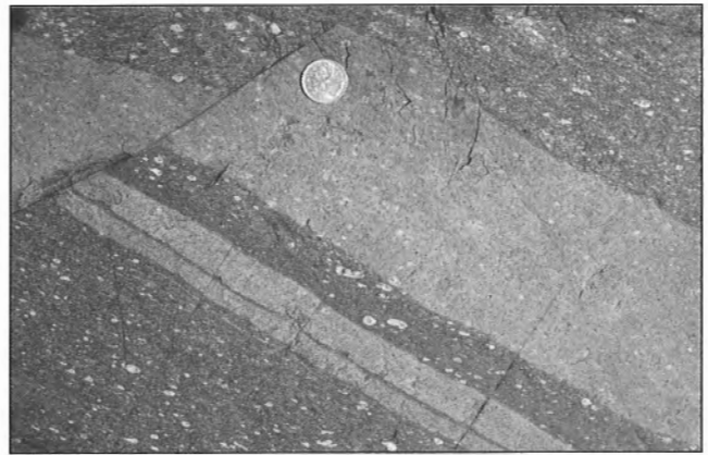
Figure 94. Porphyroclastic ribbon mylonite, Lake Athabasca west of Robillard Bay, derived from Mary granite of the type illustrated in Figure 87 (dark grey), associated with less porphyroclastic leucogranite sheets (light grey). The light grey porphyroclasts are feldspar. Coin for scale 2.5 cm. GSC 1994-220
