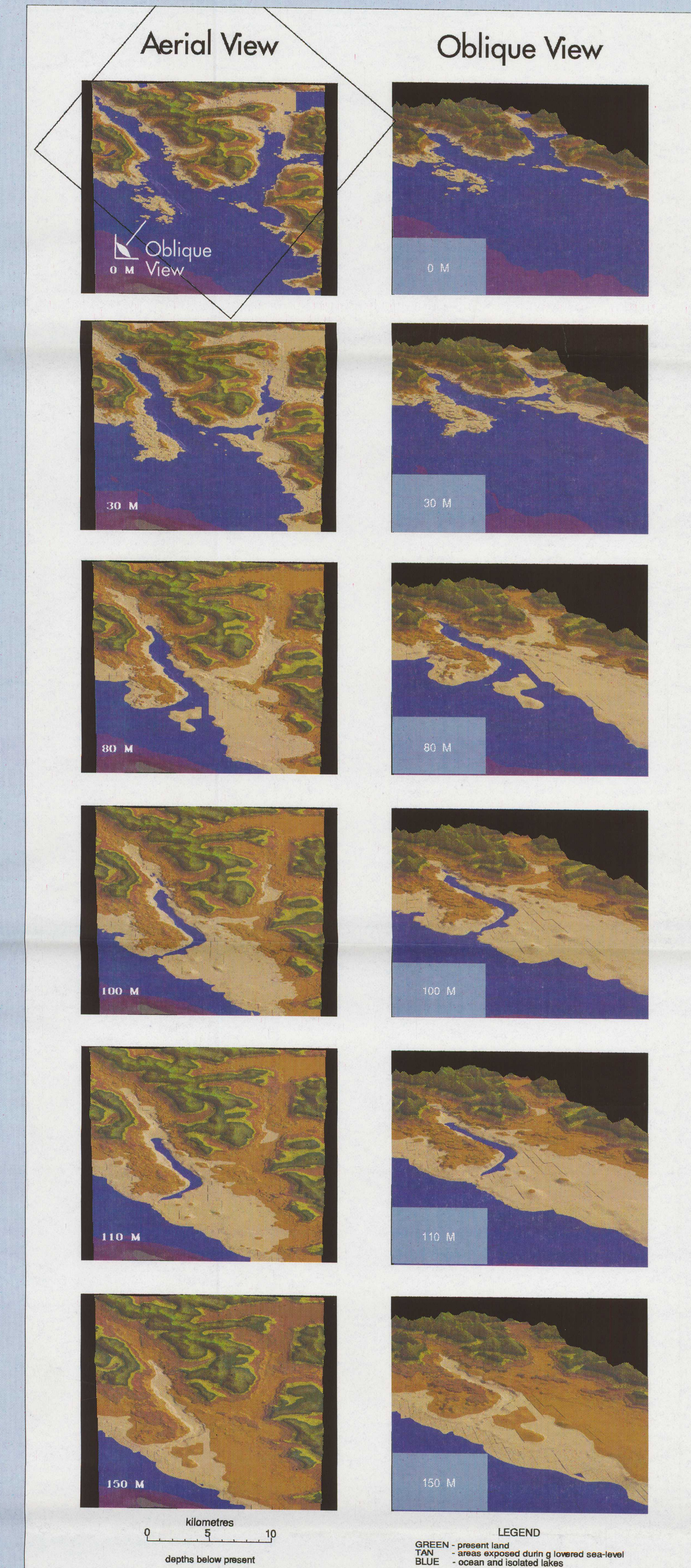
Computer generated plan and three dimensional views of study area illustrating the paleo-topography and location of paleo-shorelines during various episodes of lowered sea-levels. The terrestrial relief information is derived from 1:20 000 TRIM data set and the offshore data represents a combination of 1:40 000 nearshore navigation charts together with the 1:250 000 NRM offshore bathymetry. The data was digitally gridded and displayed by Interactive Visualization Systems.
