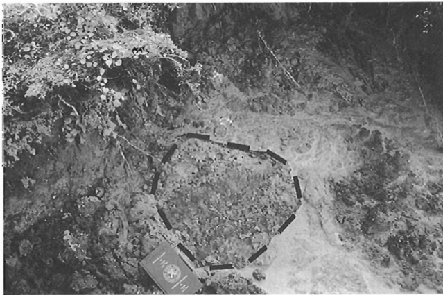
Figure 4. Ground ice in silty marine sediments. Ice (outlined) contains suspended inclusions of marine sediments and small bubble-rich pockets. GSC 1995-246H
